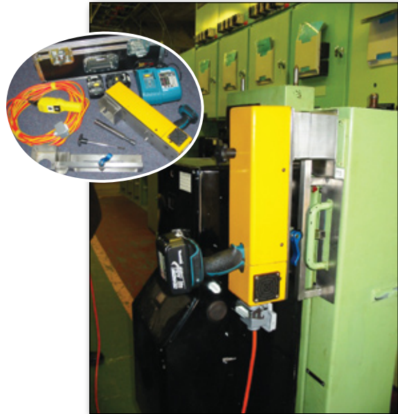
Portable remote racking unit developed by PCE allows operators to move out of the danger zone
